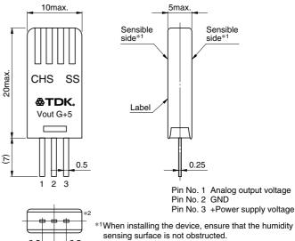
\*<sup>2</sup>The three leads are parallel to within 0.2mm.
