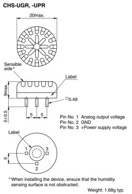
Dimensions in mm Tolerance: ±0.2
