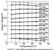
±5(%)RH specification temperature zone ----- Not specification temperature zone
