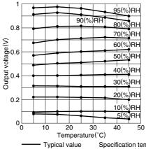
$\begin{array}{l} \mbox{Specification temperature zone} \\ +5 \mbox{ to } +45\,^\circ\mbox{C}(5 \mbox{ to } 95(\%)\mbox{RH}) \\ \mbox{Tolerance of each humidity} \\ \pm5(\%)\mbox{RH} \end{array}$
